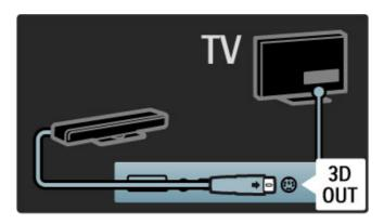
${f 3}$  Install the 3D transmitter on the top or at the bottom of the TV. Make sure to point the transmitter directly to where you sit to watch TV.
